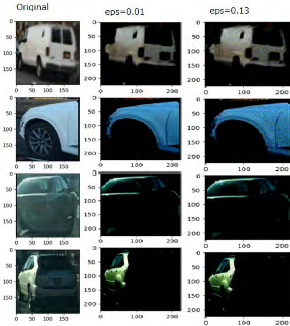
Figure 36. Data Generated Using FGSM Attack on BDD 100k Dataset for eps = 0.01 & 0.13
