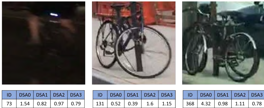
Figure 38. Bike Corner Case Examples Detected Using Surprise Adequacy
